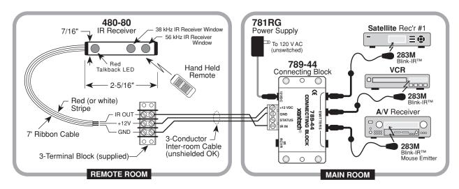
Fig. 1 A 480-80 in a basic IR repeater system.
